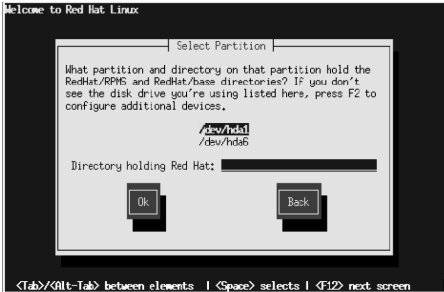
Figure 9-6 Selecting Partition for Hard Drive Install
