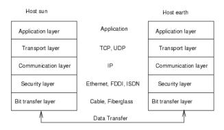
Figure 10.1: Simplified Layer Model for TCP/IP
