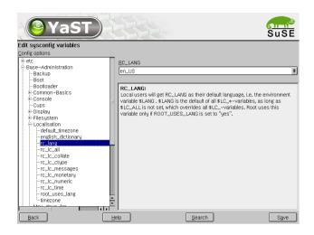
Figure 12.1: YaST2: Configuring with the sysconfig Editor
